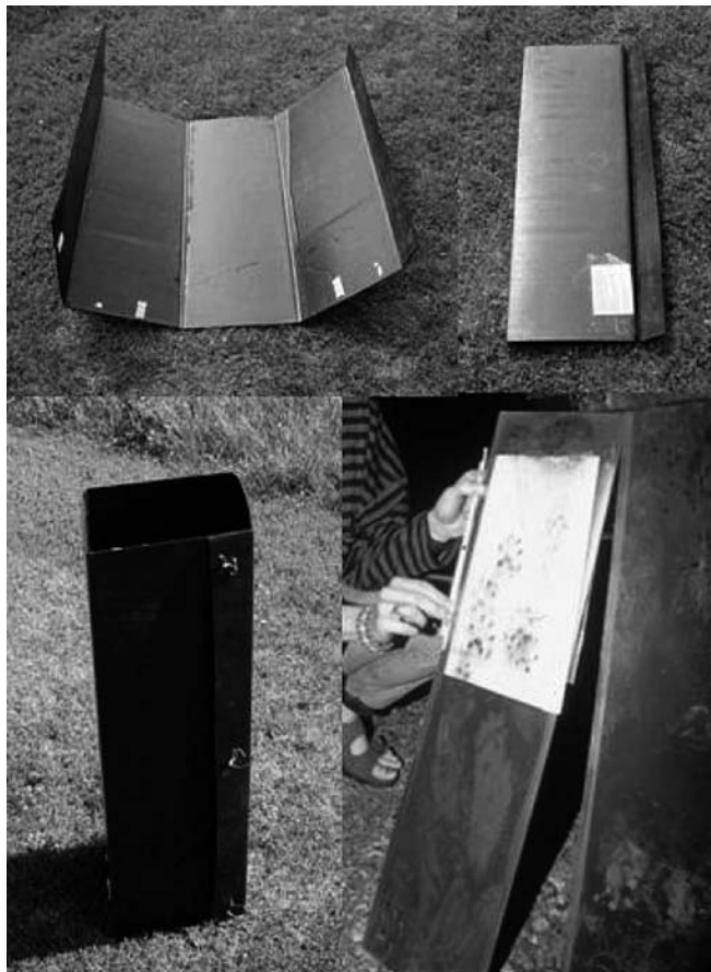
Figure 1. Enclosed track-plate design. Soot-covered aluminum track-plate is placed within corrugated plastic housing. This housing is light-weight and inexpensive and can be easily folded for transport. Bottom right displays a positive survey result from 2000 in which an Adirondack fisher has walked across the soot and left tracks on contact paper.
